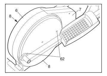
Remove the indicated Screws (62) from the Right Side Shield (7). Remove the indicated Screws (66) from both Side Shields (6, 7). Lift the Side Shields off the elliptical exerciser.
